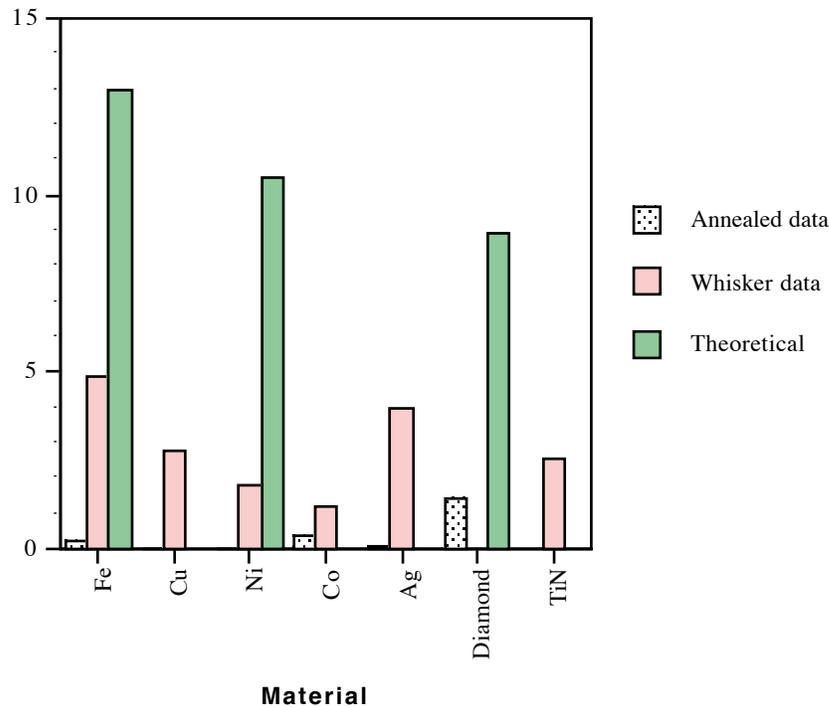
If we compare the maximum elastic strain of annealed metals and other materials with whisker data and theoretical limits, once again we see a difference of about two orders of magnitude. You may notice that the theoretical elastic strains approach the plastic strain limits of conventional materials. It is clear that while we now value materials performance improvements that are on the order of 10 or 20 percent, this isn't even close—by two orders of magnitude—to the potential of the materials.
