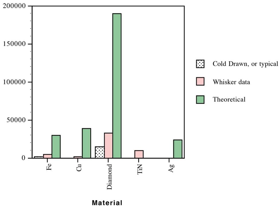
If we compare the tensile strengths of cold drawn metals and some other materials with their whisker and theoretical strengths, we see that in all cases the theoretical strengths are about two orders of magnitude greater than today's typical values.
